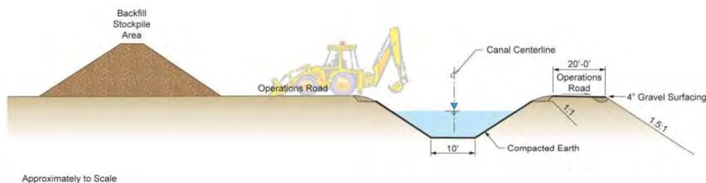
Figure 2-11. East Low Canal extension – typical cross section.
